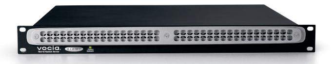
The TTS-Ince is a networked text-to-speech engine that supports the creation of browser-based announcements. The TTS-Ince uses Ethernet-based control protocols in conjunction with CobraNet® to function within a Biamp® Vocia® system and constructs announcements using a set of user-defined templates. The TTS-Ince interfaces with Rauland-Borg Nurse Call systems.
