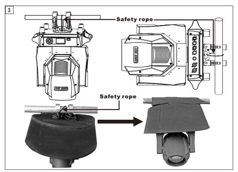
Installing the projector- Fig. 3
