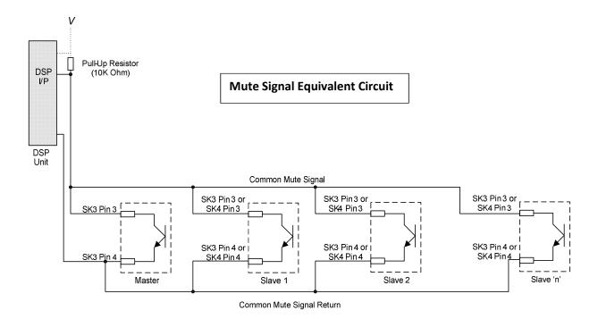
To function correctly, the common mute signal from all units must be connected via an external pull-up resistor (not supplied) to an arbitrary voltage (V) at the DSP as illustrated above. The arbitrary pull-up voltage (e.g. 5V DC or 12V DC) can either be supplied by the DSP itself (preferred option), or by an external voltage source, although if an external voltage source is used, the 0V return must be common with the DSP 0V.
