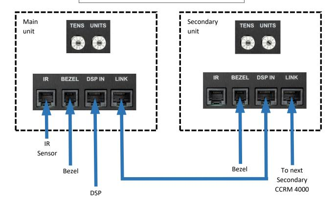
Important: When using a DSP to control the system ensure that the DSP control signal is already outputting +V to Socket 3 (DSP IN) on the CCRM 4000 Main unit (+2.5 to 12 Volts) before powering the system up. Otherwise the DSP command will not be recognised by the system and unit will fail to operate.
