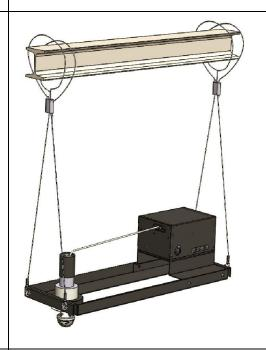
14. Push the free end of the cable harness through one of the holes located on the Gripper. Now loop the free end of the cable over a secure fixing such as a ceiling truss, eye bolt, or any structure capable of taking 7Kgs of weight. Now pass the cable through the remaining hole in the Gripper and then pull on the cable to adjust / take up the slack. Do the same with the other Y cable at the other end of the ceiling tile bracket.
