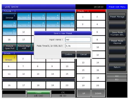
• If there is nothing on the soft-key, users can name the preset and set the fade in time. Press [Confirm] to save, the soft-key will turn to dark green. There will be a 'G' marks on the left top corner if the preset is saved by Global mode.
