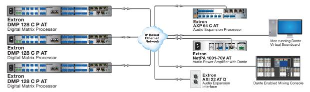
IP-based audio networking with the DMP 128 AT provides inherent scalability, allowing audio systems to be expanded simply by bringing additional processors and third-party Dante enabled devices into the network.
