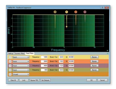
The FBS - Feedback Suppression Block is used to counteract ringing due to frequencies cycling out of control through the microphone and speakers. The feedback suppression processor for the DMP 128 engages up to twenty notch filters with adjustable Q. Fifteen of the filters are dynamic, and the processor automatically detects and then reduces the ringing. Five additional fixed filters can be adjusted manually or transferred from the dynamic filters.
