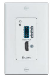
The Extron DTP R HWP 4K 231 D is a single-gang decorator-style receiver that works with Extron DTP®-enabled products to send HDMI, analog audio, and bidirectional control signals up to 230 feet (70 meters) over a shielded CATx cable. It is designed for efficient use at display locations in environments offering limited space. The HDCP-compliant receiver features a convenient one-gang form factor that offers maximum placement flexibility.
