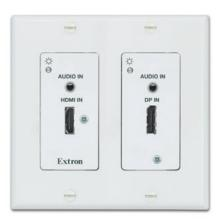
The Extron DTP T DWP 4K 232 D is a decorator-style transmitter that provides signal extension for up to two sources, sending DisplayPort or HDMI, audio, and control up to 230 feet (70 meters) over a shielded CATx cable to Extron DTP™-enabled products. The HDCP-compliant transmitter includes several integrator-friendly features in a convenient form factor that offers maximum placement flexibility.
