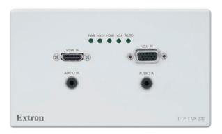
The Extron DTP T MK 232 is a two input transmitter for sending HDMI or VGA, audio, and control up to 230 feet (70 meters) over a shielded CATx cable to Extron DTP®-enabled products. The DTP transmitter is compatible with standard two-gang MK-type junction boxes for convenient installation in wall mount environments. The HDCP-compliant transmitter includes several integrator-friendly features in a convenient form factor that offers maximum placement flexibility.
