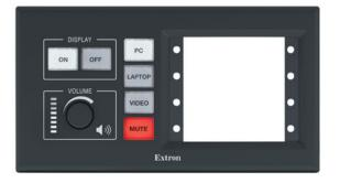
The MLC Plus 100 AAP is an easy-to-use, pushbutton controller that is for common AV room functions such as display on/off, input switching, volume, and Ethernet control of AV devices. This fully-configurable controller features a sleek look, six backlit buttons, a multi-function volume knob and an opening for four single space AAPs. It is ideal for a broad variety of AV environments, including classrooms and conference rooms.
