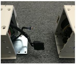
Line up modules and install joining plates
