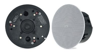
The Extron SF 3CT LP is a full-range ceiling speaker featuring a 4" deep low profile composite back can. The redesigned 3" (7.6 cm) full-range driver features a wider and smoother frequency range of 65 Hz to 20 kHz and is engineered with an extremely wide conical dispersion of 165°. The SF 3CT LP speaker is ideally suited for small to medium applications with lower ceilings and low to medium power requirements.
